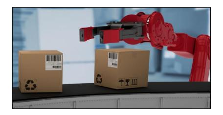
Some products may be tough for a conveyor to hit consistently in an automated set-up, perhaps due to an irregular surface, a complex shape, or other logistics. An engineered semi-automatic design may be optimal for expense as well as production needs.
